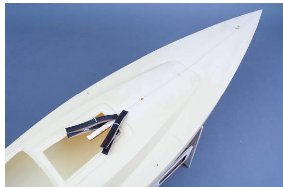
Fig. reinforcing board in position
