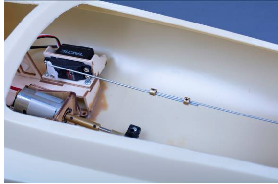
Fig. servo mount with servo
