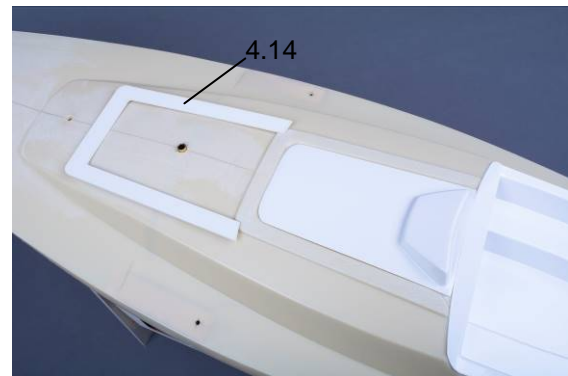
Fig. sliding hatch and frame
