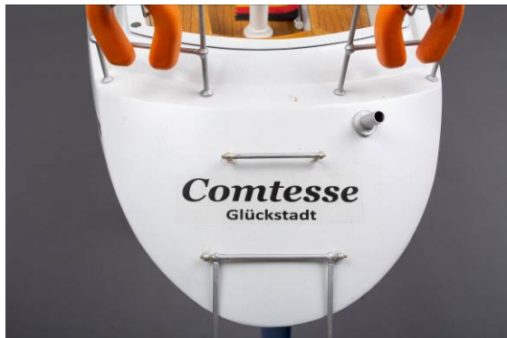
Fig. bathing ladder folded down, additional rung
