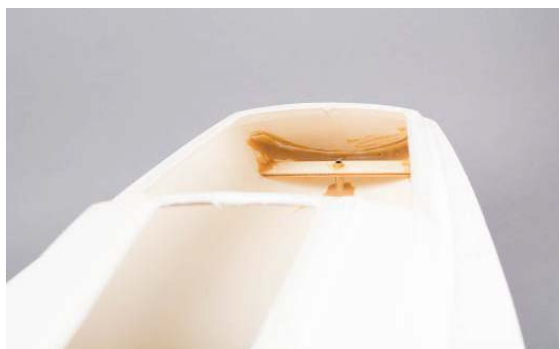
Fig. glued rudder bearing
