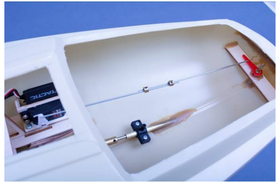
Fig. connection servo and rudder
