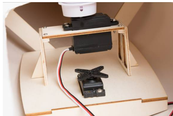
Fig. Sail winch frame on RC board
